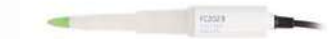
FC2023 Open viscolene reference electrolyte, double junction, PVDF body pH electrode with conical tip and temperature sensor Recommended for dairy analysis including cheese, yogurt, and other semi-solids
