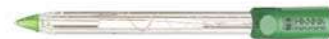
HI10533 Triple ceramic, double junction, glass body, refillable pH electrode with conical tip and temperature sensor Recommended for fats, creams, soil and low conductivity samples
