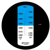
The MASTER-URC/N $\alpha$  is designed to quickly and easily measure Urine Specific Gravity with just a single drop of sample. The new plastic body design is resistant against corrosion from salty and acidic samples, and incorporates an improved optics system for higher contrast and better clarity. Simple to use, lightweight, and portable! It is featuring a water resistant design and Automatic Temperature Compensation.
