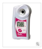
PAL- cleaner is a model that can be measured with high resolution of decimal two digits of 0.01%. This is ideal for measuring low concentration of the solution, such as industrial cleaning fluid.
