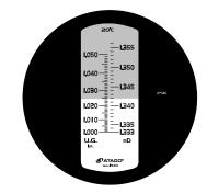
● Left side scale : Indicate specific gravity of urine.
