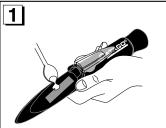
Put one or two drops of sample on the prism.
