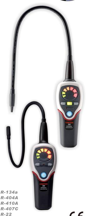
CENTER 380/382 is a perfect tool for air-condition system maintenance. The operation interface is intuitive with buttons, light bar and sound. The "air sucking system" (382) greatly helps the sensitivity and response time. The "auto-reset" (382) function can help the operator to distinguish the leaking spot among the already spreading refrigerant while maintaining high sensitivity.
