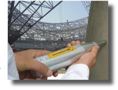
With the merits of simple structure, easy correction, maintenance and repair, and portability, the concrete test hammer is widely used in civil engineering and construction industry for testing the strength of concrete.
