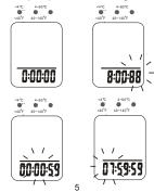
Press MEAS to start countdown with previous setting, or press SET button to have a new one. The Second digits will blink first for value change. Press SET again to increase the value and then MODE to select minute and hour digits. After hour setting is completed, press MEAS to count down.
